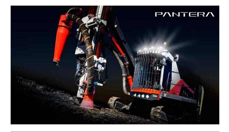
PANTERA<sup>™</sup> DI6400 is an advanced high-pressure DTH drill designed to meet the mining industry's future needs in terms of safety, increased production and full automation options. It is designed for vertical and inclined drilling of 115–203 mm diameter blastholes up to 45 meters deep, for wall control, pit development and production drilling.
